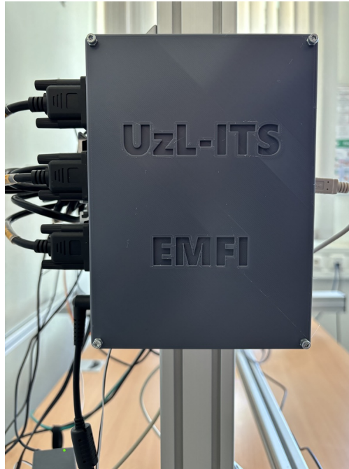
Figure 9: Stepper controller with DB9(M) stage connectors.
