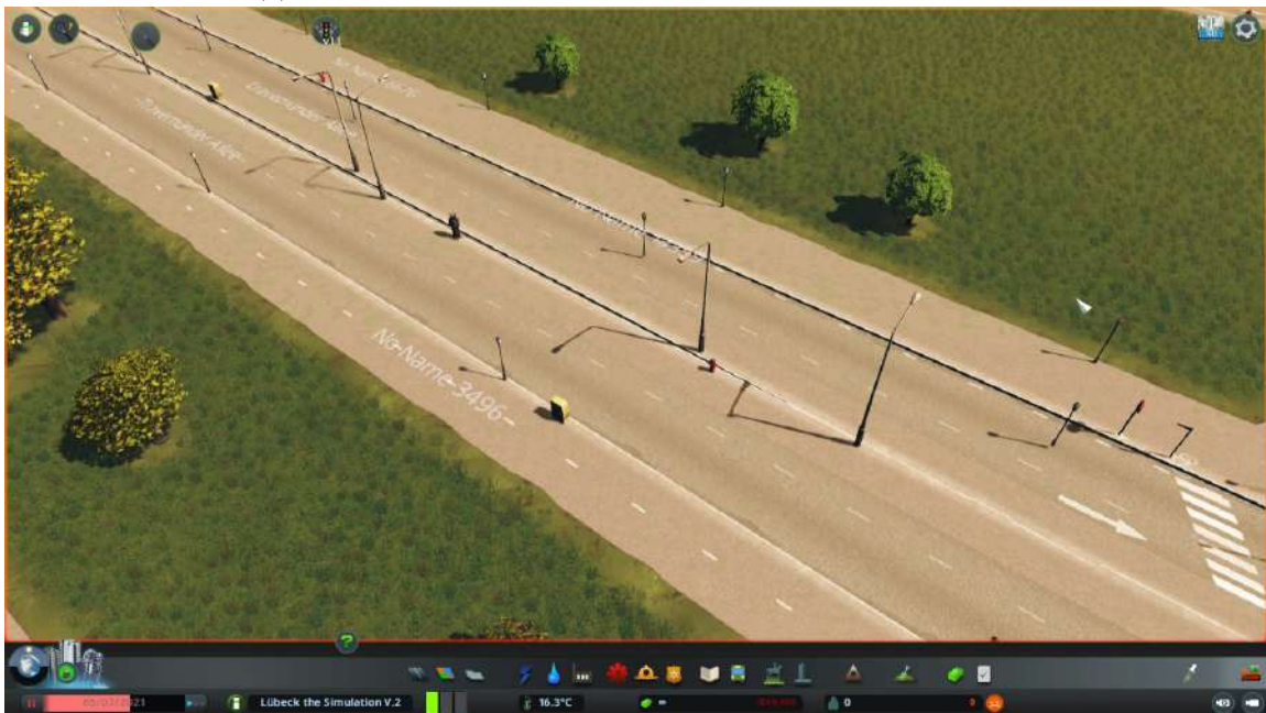
(b) Normally these two streets would be deemed "too close" to each other, but because the mod sets them down in one instantaneous moment this limitation does not apply. If one was to delete one of these streets however they would not be able to place them down again.
